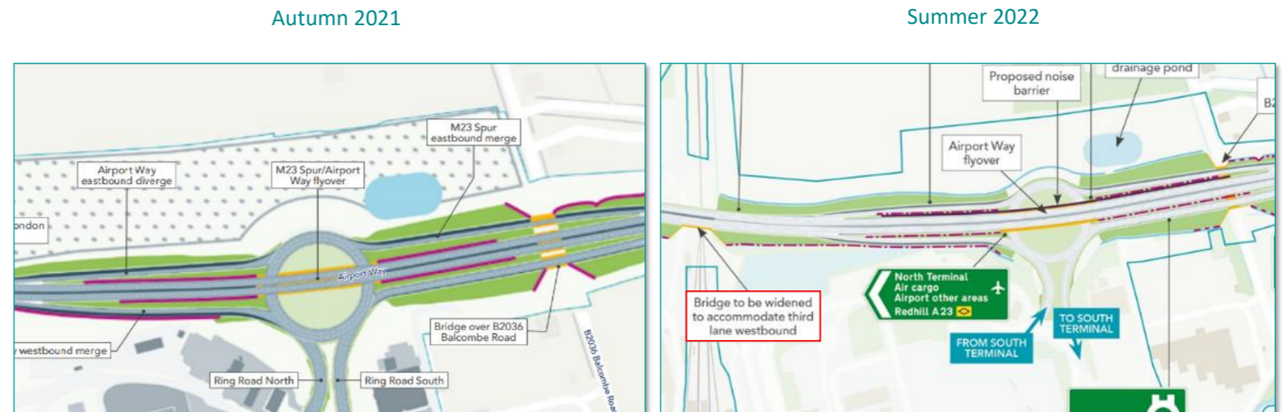
South Terminal junction largely unchanged but westbound slip from South Terminal now a lane gain arrangement to avoid traffic weaving. This requires widening of the bridge over the Brighton mainline railway
